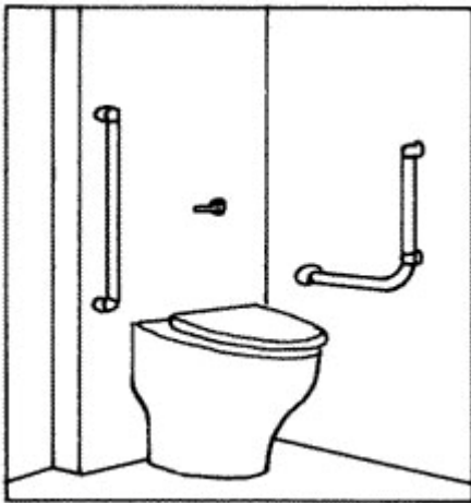
Figure 13 Side and back mounted bars.
